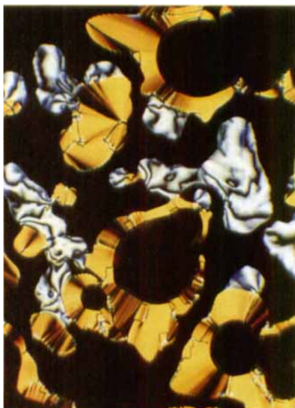
Figure 4. Smectic C phase of I-C 16 emerging from the isotropic phase ( T=290^{\circ}\text{C} ).
